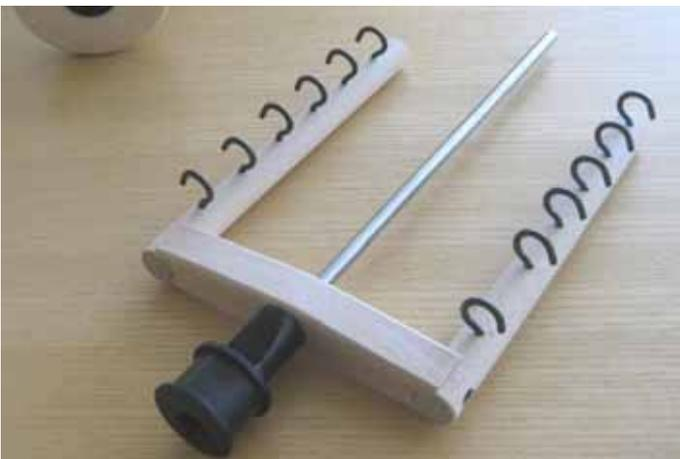
Screw the 12 hooks into the flyer, using the pre-drilled holes. The hooks need to be completely screwed into the flyer, up to where the bend starts.
