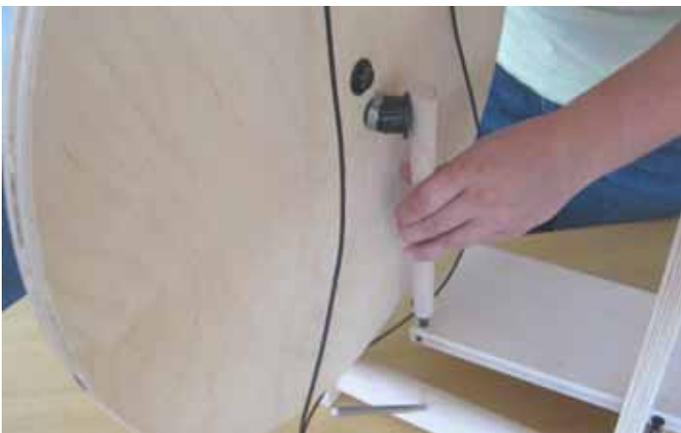
Snap the nylon cup over the ball bearing on the wheel. Make sure the drive band is between the wheel and the footman. Secure the connection by sliding the ring towards the wheel, until it is on the edge on the cup.
