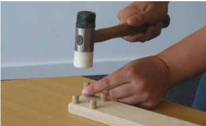
Tap the four wooden dowels into the holes at the bottom of the front post.
