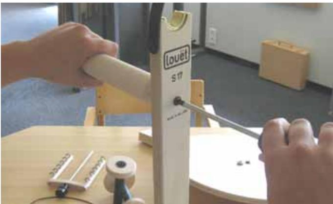
Take the shortest of the four large screws and screw the front post onto the end of the second round bar.
