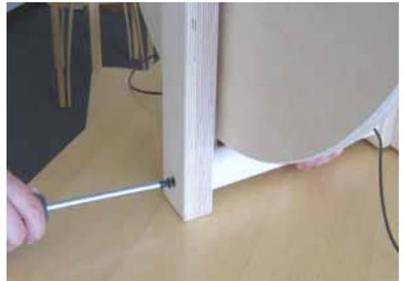
Use the other two screws to assemble the back post. Lead the drive band through before you make the last connection.
